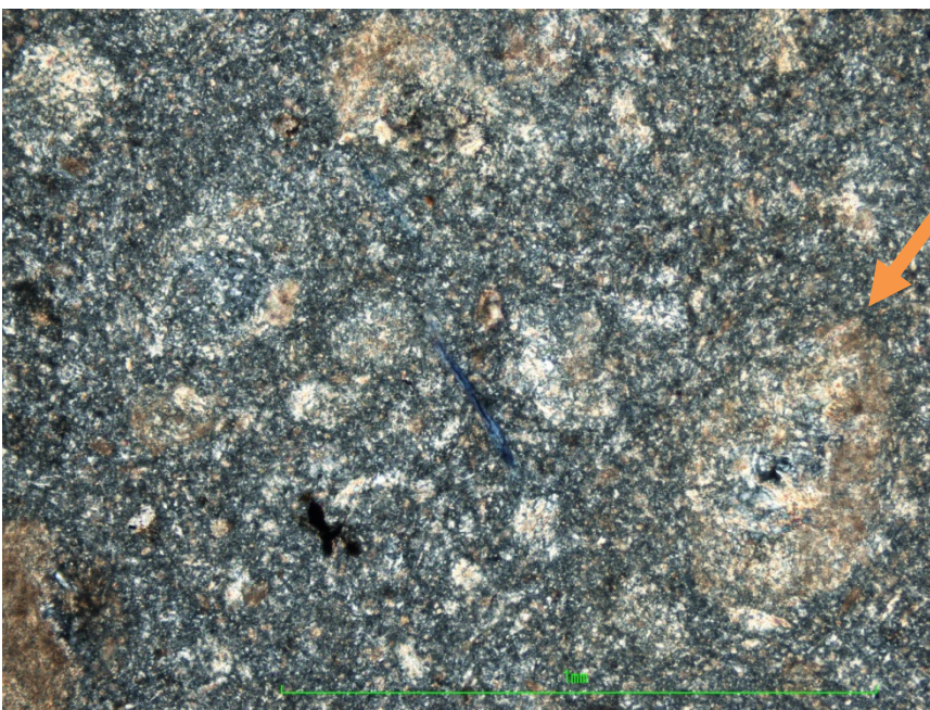
Figure 3. This thin section was taken from a gypsic horizon (10-20 cm depth) and shows a lenticular gypsum crystal, which is disintegrating as a result of pedogenic processes (arrow).
